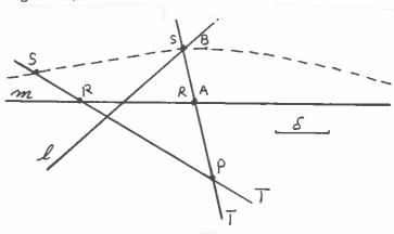
an adjustable pin R ot it. The pin is adjusted such that RS =  $\delta$ . Then the ruler is made to slide along the given point P while the pin R is guided along the line m. The movement is stopped the moment that S coincides with  $\ell$ ; SR is then the required position for the segment AB.
