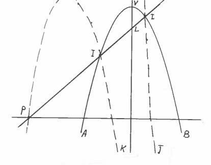
The parabola AVB moves in vertical direction along its axis. The straight line PL turns around the fixed point P and is linked to the parabola in such a way that its intersection L with the axis keeps constant distance from the vertex V. The intersections I then trace the "Cartesian parabola" PIK, HIJ. As the parabola itself is acceptable in geometry, the "Cartesian parabola" is also acceptable.
