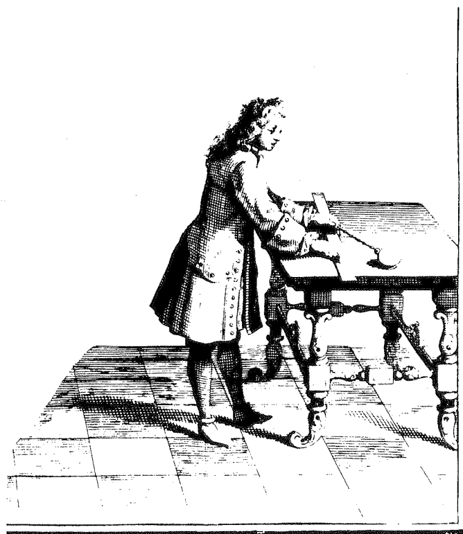
Fig. 26 Tracing a tractrix by means of a chain watch, from [Poleni 1729].
